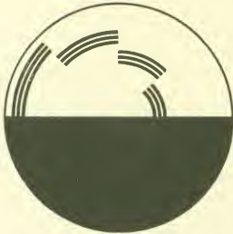
Fig. 67. — By rotating this Mason (black and white) disk color-sensations are produced.
