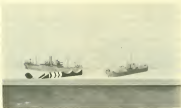
Figs. 95 and 96. Illustrating the use of models by the Navy Department in developing the geometrical-illusion for ships.
